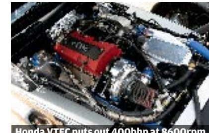
Honda VTEC puts out 400bhp at 8600rpm
