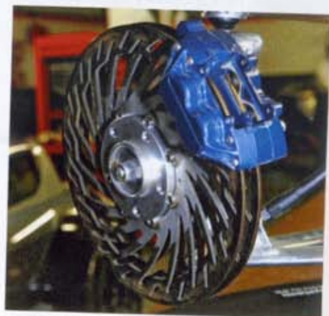
Above: twin-disc brakes are just one of the new technologies from IFR being showcased on the Aspid
